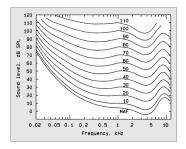
sound pressure required for a test tone of any frequency to sound as loud as a test tone of 1 kHz
